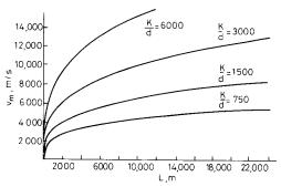
Fig. 6 Sensitivity of  $v_m$  to d and k
